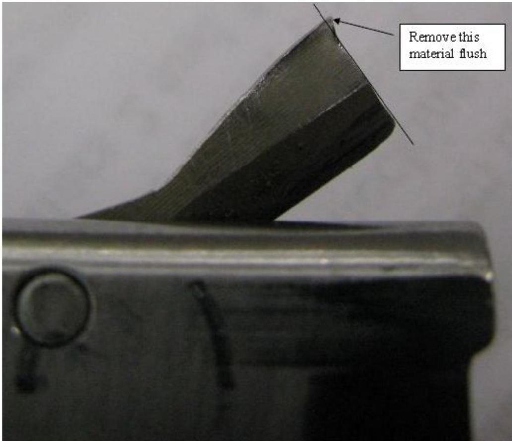
When the tool is set up correctly the backside end of the cutting blade does not contact the external tool body. If the internal tool body is set too deep inside the external tool body wear as depicted in the above picture will occur. The raised material shown in the picture must be removed with a stone or by sanding to prevent damage to the aircraft structure during use. Take care not to remove material near the cutting surface of the blades.
