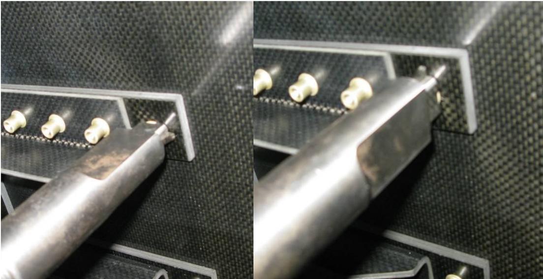
Ensure there is sufficient clearance of the outer body to surrounding parts to prevent damage to structure during the cutting process.
