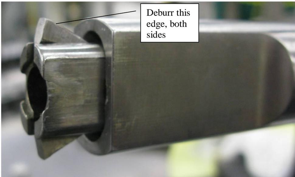
As the cutting blades wear they may begin to stick in the blade slots. The blades should be deburred on the backside that contacts the outer housing to restore original functionality. The cutting surfaces of the blades should be inspected frequently and replaced when dull. The cutting blades should also be replaced when multiple cuts are required to relieve the tension of the collar, providing the tool is in proper adjustment.
