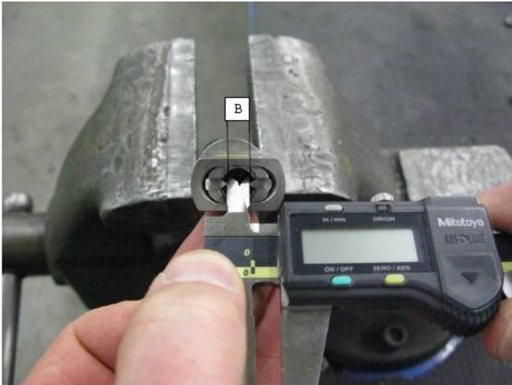
Dimension B, distance between cutting blades when internal and external tool bodies are flush. If dimension B is below the recommended values in the table readjust tool bodies. If dimension B is beyond the recommended values in the table replace the cutting blades. Do not adjust internal body below flush to the external body to achieve proper setting of dimension B except in extreme emergency cases. *Improper setting of this tool can result in damage to the aircraft structure.*
