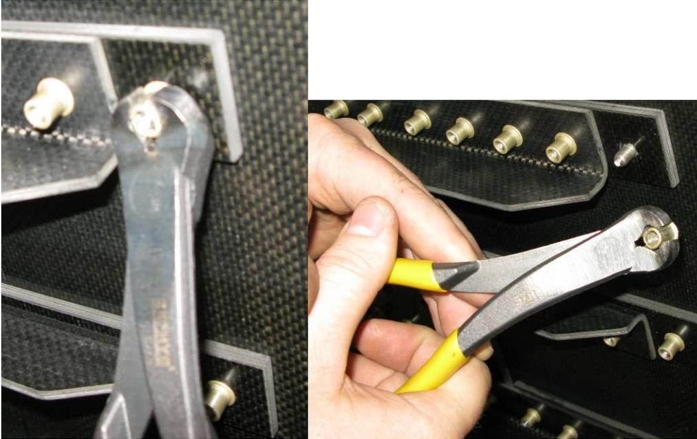
The collar can be removed with standard Hi-lok pliers. Take care not to grip to the collar too tightly with the pliers, as this will potentially make the collar more difficult to remove. Once the collar is broken free with the pliers the collar can typically be unthreaded by hand.
